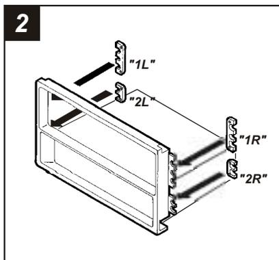
Attach **Spacer 1L** and **2L** to the left mounting tabs of the **Radio Housing** and **Spacer 1R** and **2R** to the right mounting tabs of the **Radio Housing** as shown. Skip to the *Installation Instructions for ALL VEHICLES* on Page #3.
