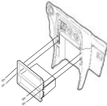
Re-connect the battery terminal and test the unit for proper operation. Mount the head unit/kit assembly to the sub-dash with **(4) #10 x  $\frac{3}{4}$ " Phillips Truss-head Screws** supplied.
