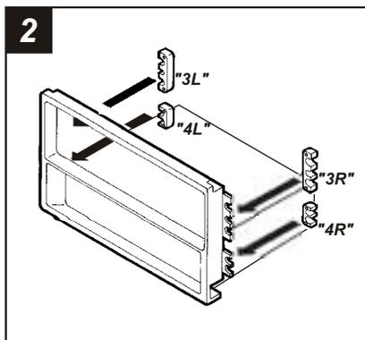
Attach **Spacer 3L** and **4L** to the left mounting tabs of the **Radio Housing** and **Spacer 3R** and **4R** to the right mounting tabs of the **Radio Housing** as shown. Skip to the *Installation Instructions for ALL VEHICLES* on Page #3.
