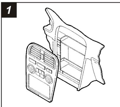
Disconnect the negative battery terminal to prevent an accidental short circuit. Detach the cable located under the left side of the glove box. Unclip the trim piece in front of the gear shifter and remove (2) Phillips screws exposed. Unclip the gear shifter trim and remove (2) Phillips screws exposed. Unclip the radio trim bezel and remove. Remove (6) Phillips screws securing the factory head unit and disconnect the wiring.
