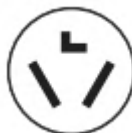
3-wire receptacle (10-30R)
