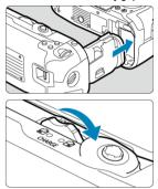
Insert the battery grip in the camera and turn the release dial to lock it in place.
