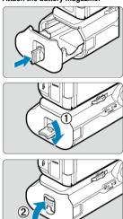
Insert the battery magazine all the way in to secure it.
