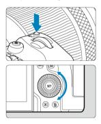
Press a button such as  $\langle M-F\eta \rangle$ , then turn the  $\langle 0 \rangle$  dial.
