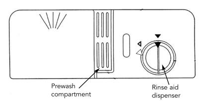
**NOTE:** The dishwasher has an indicator on the control panel that displays when the rinse aid dispenser is almost empty. After refilling the dispenser, there may be a small delay before the indicator goes out.
