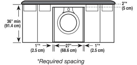
\* Most installations require a minimum 5" (12.7 cm) clearance behind the dryer for the exhaust vent with elbow. See Installations Instructions, "Venting Requirements."
