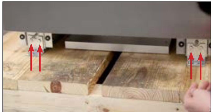
FIG. 7. Shipping bracket bolt locations.
