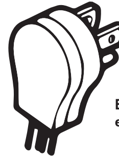
Power supply cord with 3-prong grounding plug
