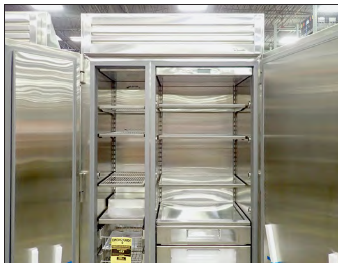
FIG. 7. Completed shelf installation.
