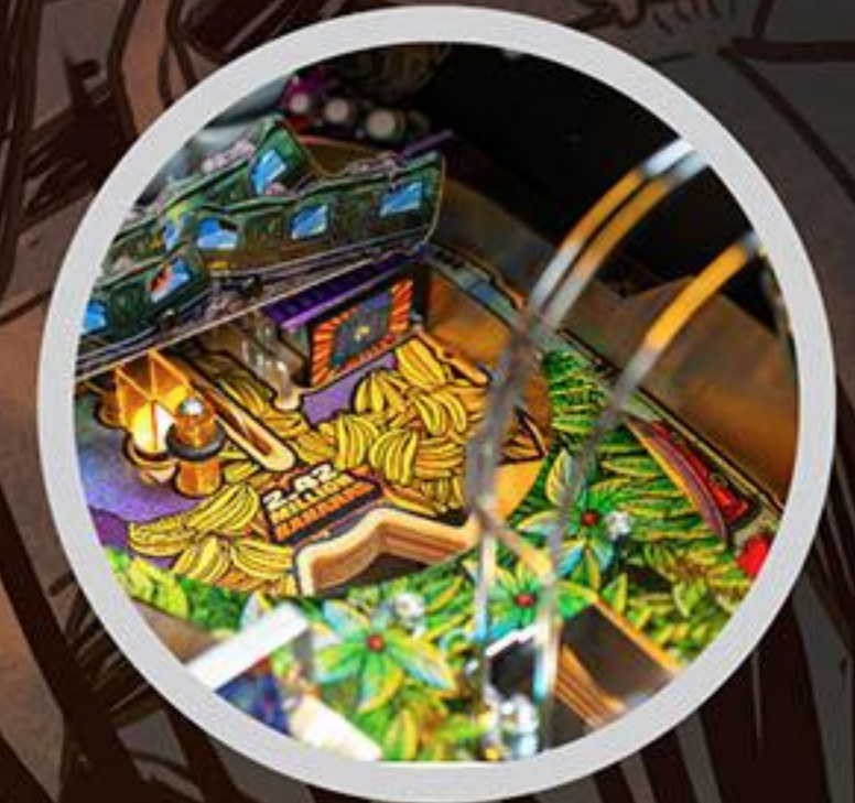
Survive Kong's punch-back kicking target which launches balls back at the player or can drop balls into secret entrance to Kong's VUK and wireform return.
