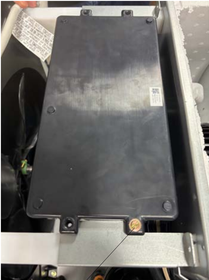
Remove top screws (4 places)
