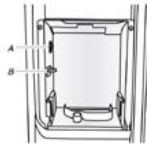
A. On/Off switch B. Storage bin sensor
