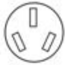
3-wire receptacle (10-50R)
