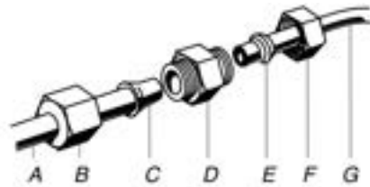
A. Refrigerator water tubing B. Nut (provided) C. Bulb D. Coupling (purchased) E. Ferrule (purchased) F. Nut (purchased) G. Household water line
