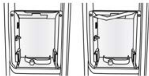
Ice production Off (shut-off arm up)
