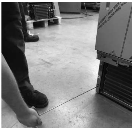
Adjusting front leveling legs.
