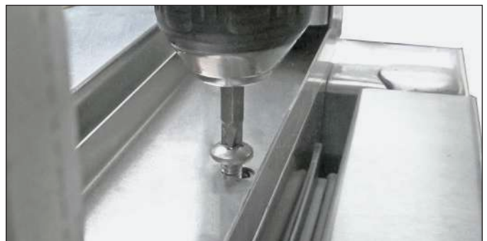
FIG. 10. Remove the screws from the metal channel.
