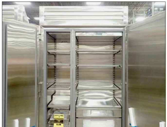
FIG. 7. Completed shelf installation.
