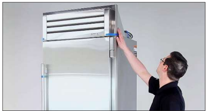
FIG. 2. Inspect the unit's exterior for visible damage.
