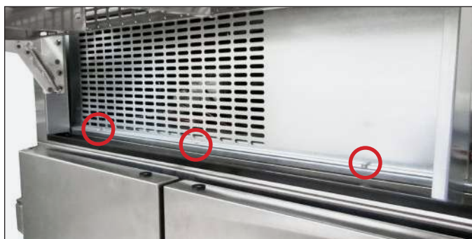
FIG. 9. Rainshield screw locations.
