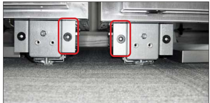
FIG. 11. Remove and discard the interior magnet brackets.
