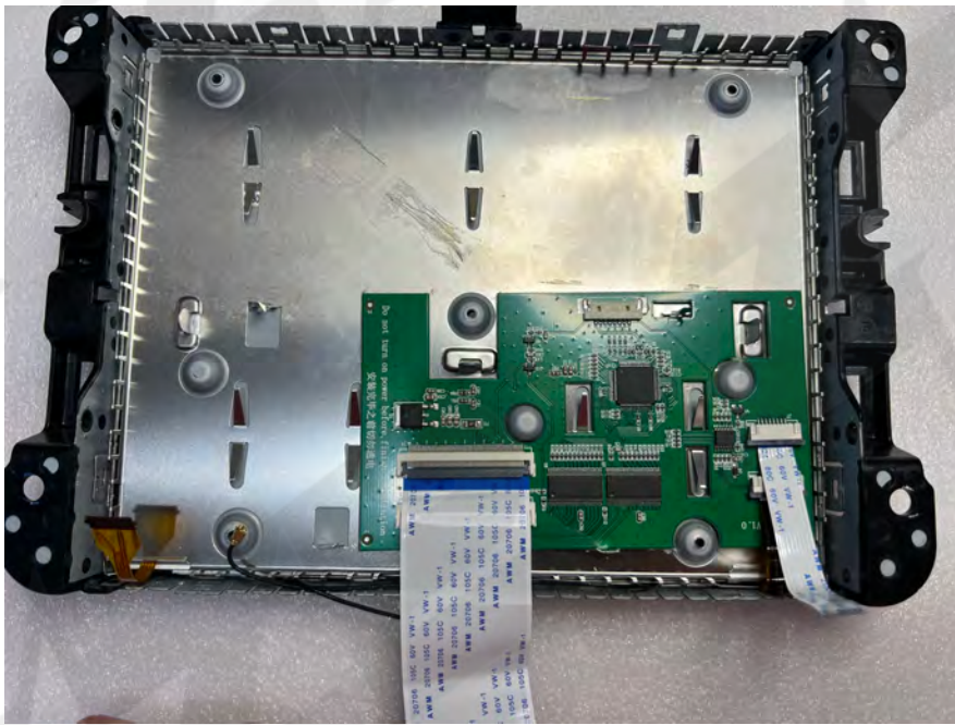
12. The PCB should look like this when connected properly.
