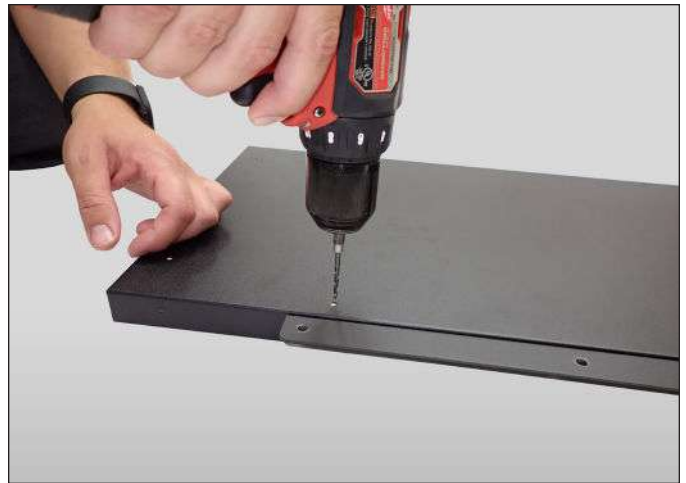
FIG. 4a. Drill pilot holes through the drawer front assembly.
