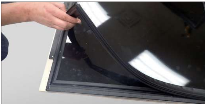
FIG. 3. Pull the gasket from the door.
