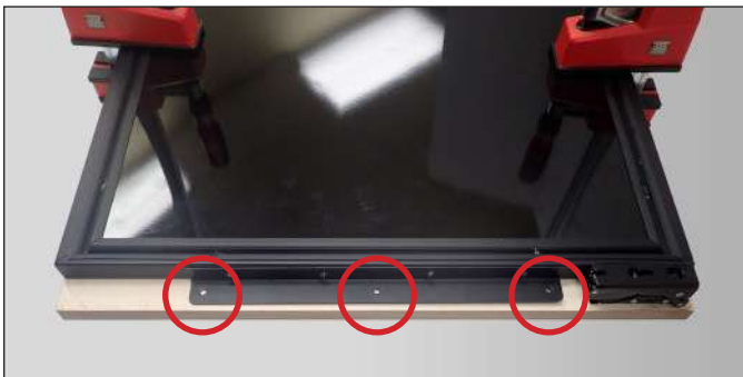
FIG. 5. Carefully drill pilot holes in the panel.
