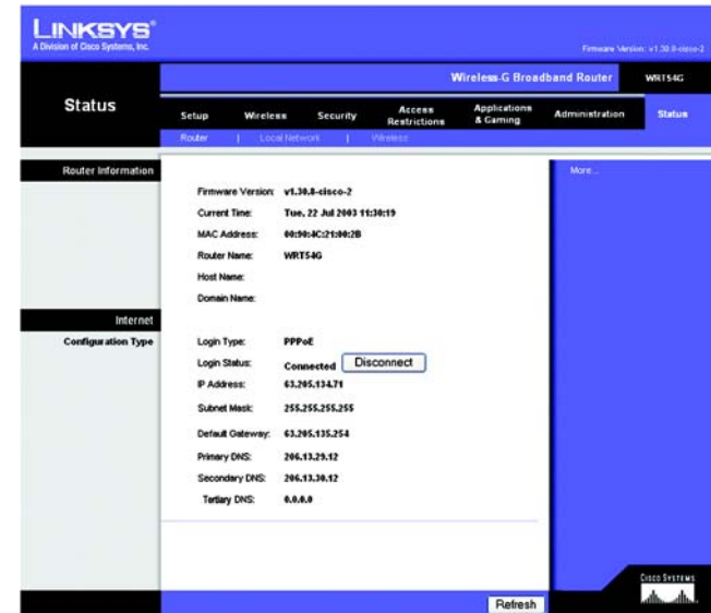
Figure 5-46: Status Tab - Router
