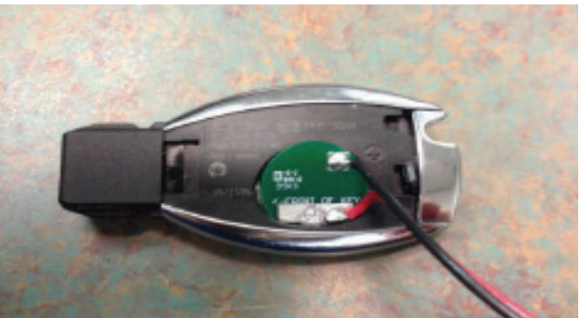
Insert battery emulator- bottom first
