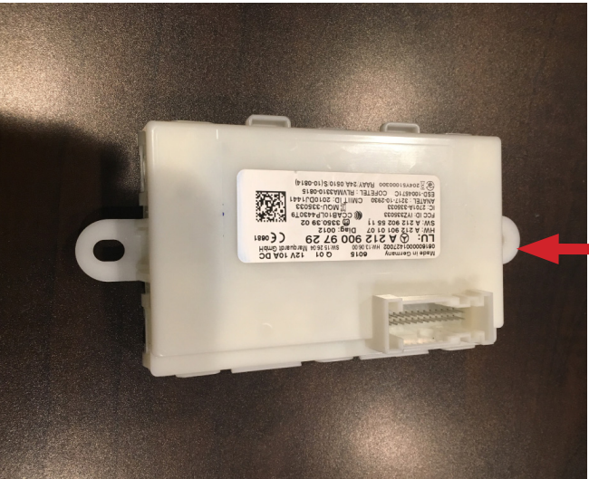
Note: 2014+ w166 KG module has slightly different plug configuration (pictured)
