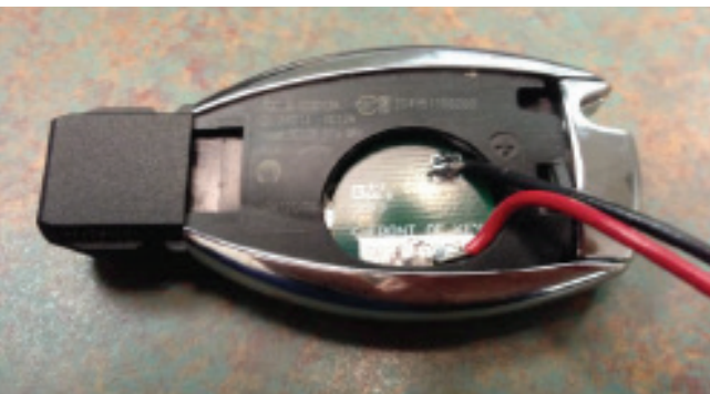
Push battery emulator fully into place
