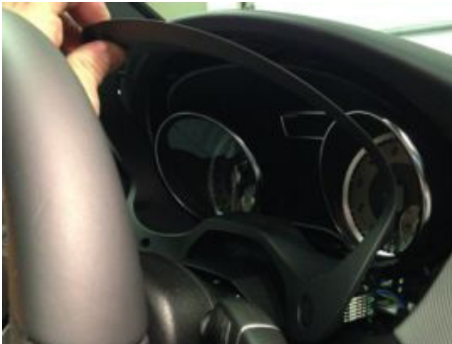
Remove bezel and unplug HVAC sensor
