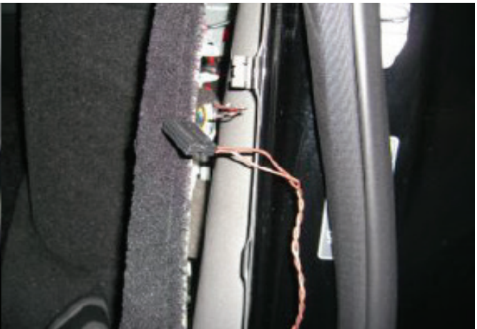
KG harness properly installed into plug
