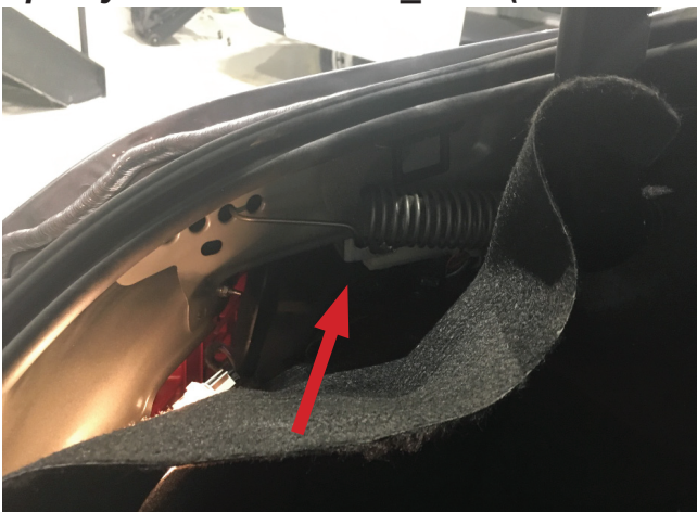
Remove carpeting and access wire trough
