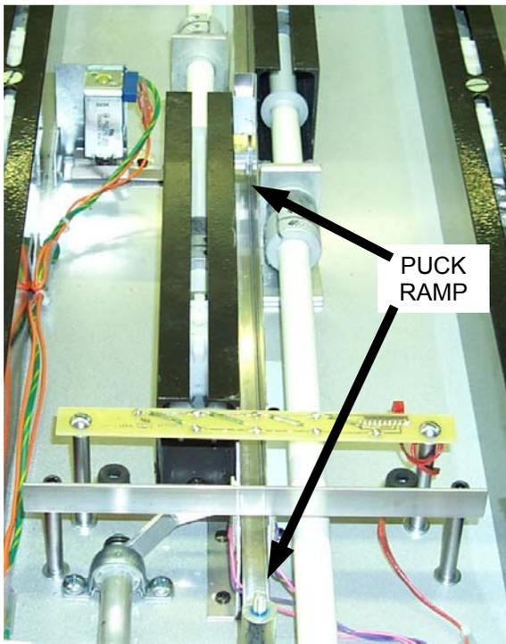
3. A puck ramp may become pushed up during shipping or moving. Just push it back down in the retainer/chute with a pencil or screwdriver.
