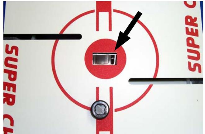
2. To determine if the ejector is misaligned, first remove the ice surface and then start the game. Look straight down the ejector chute and observe how the puck ejects. If the puck consistently hits one side of the chute, the ejector should be adjusted. Loosen the 2 screws that mount the solenoid assembly to the cabinet. Re-position the assembly so that the cup where the puck sits is centered into the vertical area of the chute.
