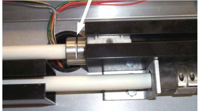
collar make sure the rod and gear box coupler touch, and retighten the gearbox. Be sure to leave 1/32" to 1/16" between the collar and the gearbox body.
