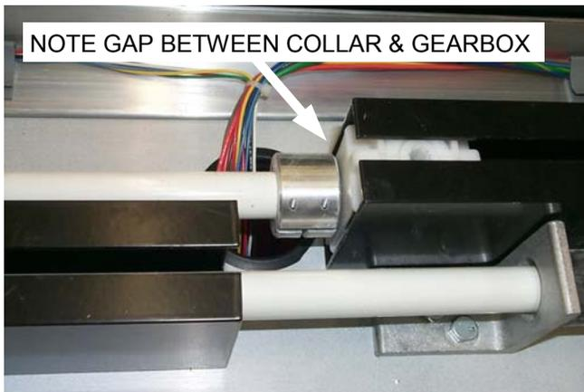
**NOTE GEARBOXES ARE LUBRICATED FOR LIFE AND SHOULD NOT BE OILED OR GREASED.**
