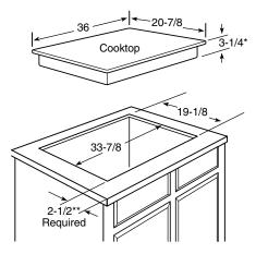
\*Depth of unit at conduit connection location (rear) is 6-1/2" on models PP980/950 and 4-5/8" on models PP975/972/962/945/942/932/912, JP655/356/346.
