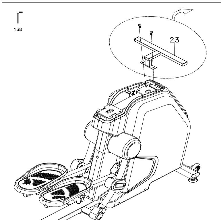
1. Use L Allen Wrench (No.138) to remove two  $3/8'' \times 3/4''$  Socket Head Cap Bolts that hold the protective Side Back (No.23) onto the mounting plate on the Main Frame. Discard the bolts and set the Side Back (No.23) aside.
