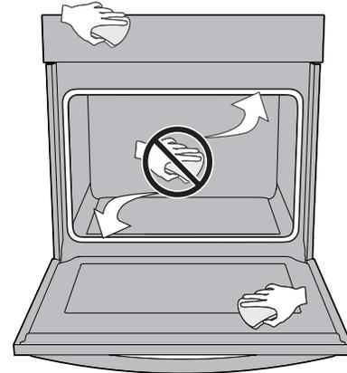
**Figure 13: Clean around the oven door gasket**
