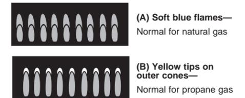
Long, bright yellow flames are not normal. Normal flames may show signs of an orange tint when well heated or signs of flickering orange due to particles in the gas or air.
