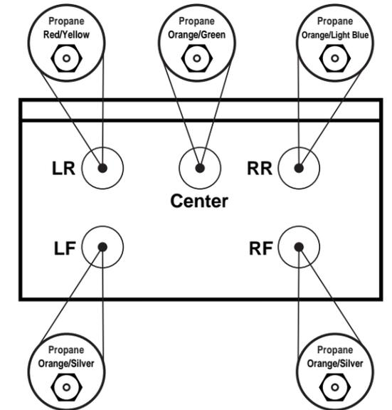
To prevent leakage, make sure the orifice spuds are securely screwed into the gas supply tubes.
