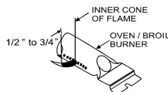
**NOTE:** If burner flames look like (A), further air shutter adjustment to the bake burner is required. Normal burner flames should look like (B) or (C), depending on the type of gas you use. With propane gas, some yellow tipping on the outer cones is normal.
