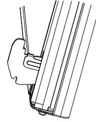
4. Open the door completely and unlock the hinges.
