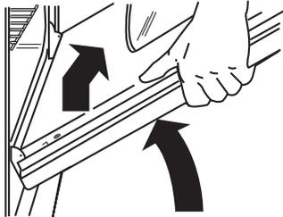
3. Pull door straight up, then toward you. Do not unlock the hinges until the door is replaced on the range.
