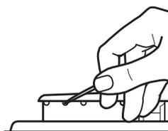
5. Replace the burner cap, making sure the alignment pins are properly aligned with the burner cap.
