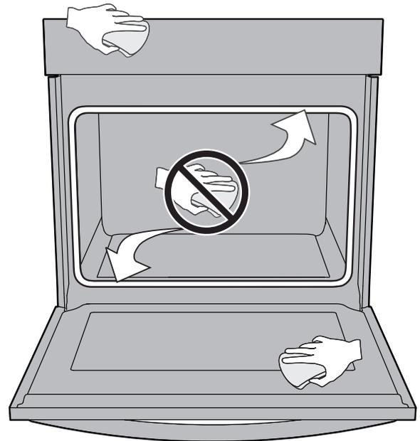
**Figure 4: Clean around the oven door gasket**
