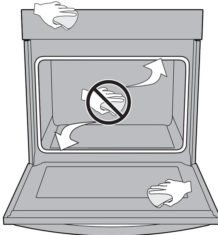
**Figure 6: Do not clean oven door gasket**
