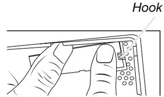
6. Reattach the second top vent cover with the screw removed in step 1.
