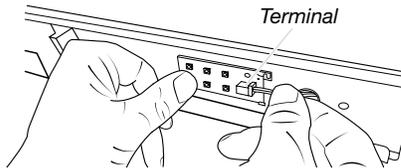
4. Replace a new LED, press it back between two hooks and plug in the terminal.
