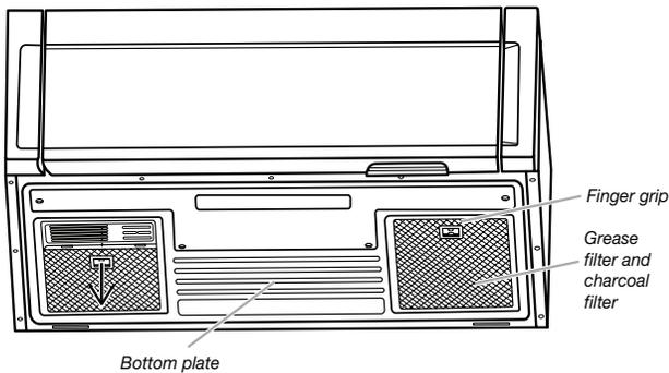
2. Clean the grease filter monthly, or replace with new grease filter if necessary.
