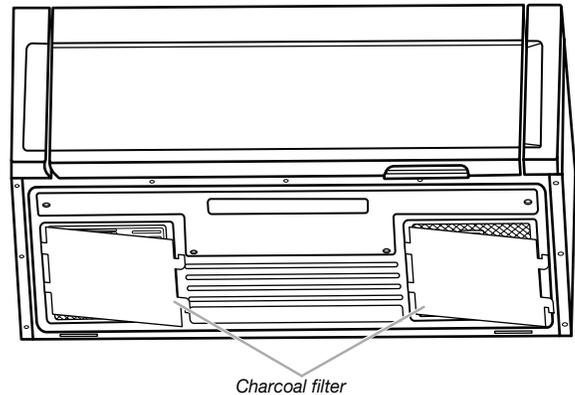
3. Replace a new charcoal filter and reattach it back to the bottom plate, and make sure both left and right sides insert to the bottom plate slots.
