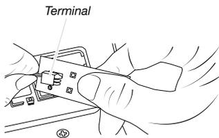
5. Replace a new LED, and snap it into the hook.
