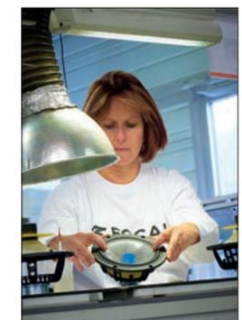
Assembling the new *Sopra* midrange driver on our *Ariane* production line. Based on the principle of lean manufacturing, we employ highly-qualified workers who have completely mastered every step of the procedure from start to finish.
