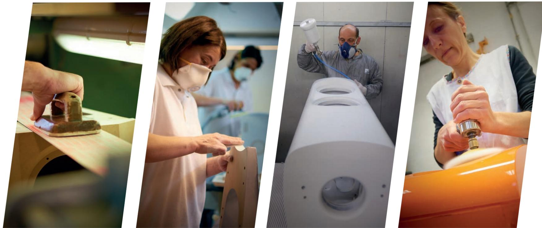
The front baffle is machined from a 2" (69mm) sandwich of MDF using the "Gamma Structure" principle. Its density is substantial enough to exploit the mechanically inert structure for maximum definition.
