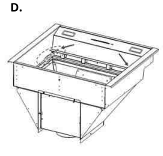
Figure D: Remove Control Panel Remove screws (front and back) attaching panel to ventilation hood liner.
