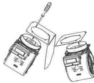
Figure C: Connect Blowers Install dual 600 CFM blowers onto hood with included hardware. Connect molex connectors to blowers.
