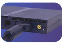
Connect the flat end of the RFU Adaptor to the AV MULTI OUT connector on the back of the PlayStation 2 system.
