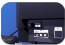
Connect the RFU OUT connector to the cable connector on the back of your TV. This is where you ordinarily connect your coaxial cable for an antenna, cable TV, or VCR. Plug the cable into the area marked ANT on the RFU adaptor.
