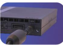
Connect the AC adaptor to the AC power cord. Connect the AC adaptor end to the PlayStation 2 system.
