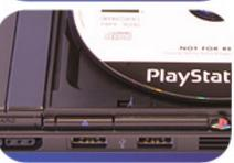
Press the open button on the front of the console and set a disc in the disc holder. Press down gently on the disc until all three tabs on the disc holder are above the surface of the disc. Press the "PUSH" label on the disc cover to close it.
