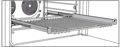
The FlexiClips with Wire Rack are mounted on the side racks and can be pulled completely out of the oven. This allows you to see the food easily.
