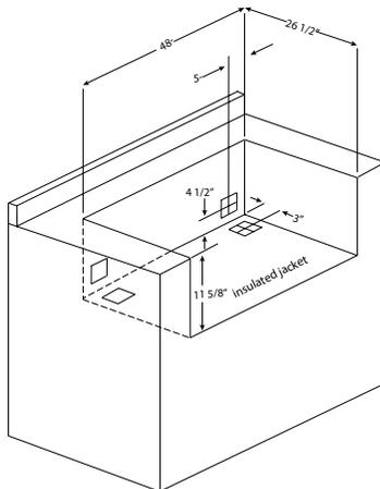
4" square holes for gas and electrical connections both left and right sides (rear or bottom access). Make these holes in the frame based on your requirements. 120V GFI outlet must be located within 6' of the 4" hole.
