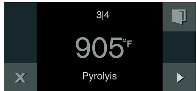
A signal sounds once the pyrolytic self-cleaning function has ended. A message appears in the display. Once the appliance has cooled down, wipe out the ash that has been left behind in the oven cavity with a damp cloth.
