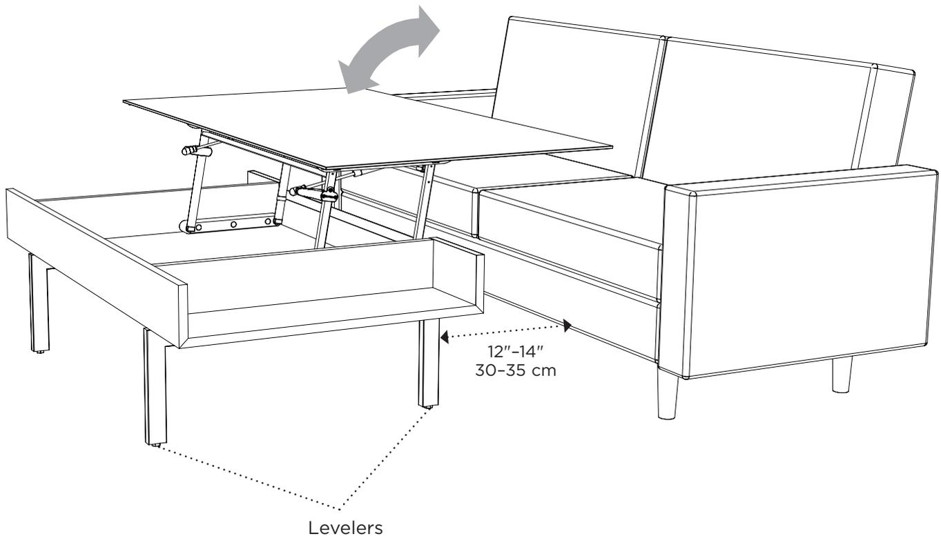
The preinstalled **(H3) Nylon Levelers** are intended for use on carpeted surfaces.
