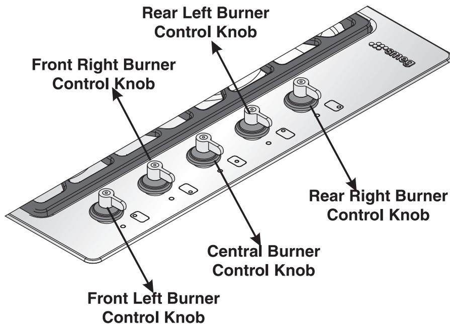
**Use the front left and the front right burners** for simmering or for cooking smaller quantities of food requiring small cookware.
