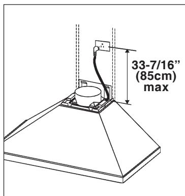
Set the electrical power supply within the space covered by the decorative flues. Position an electrical outlet at a maximum distance of 33-7/16" (85 cm) from where the lead exits from the hood (see illustration alongside). Make sure this does not interfere with the decorative flues (where the flue touches the wall).
