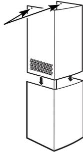
The inside duct piece must slip into the folded ends of the outer section.
