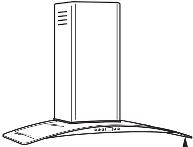
**NOTE:** Measure installation height from the cooking surface to the outer glass portion of the hood.
