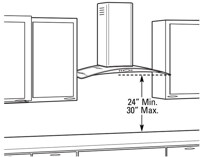
**NOTE:** Installation height should be measured from the cooking surface to the outer glass sides.
