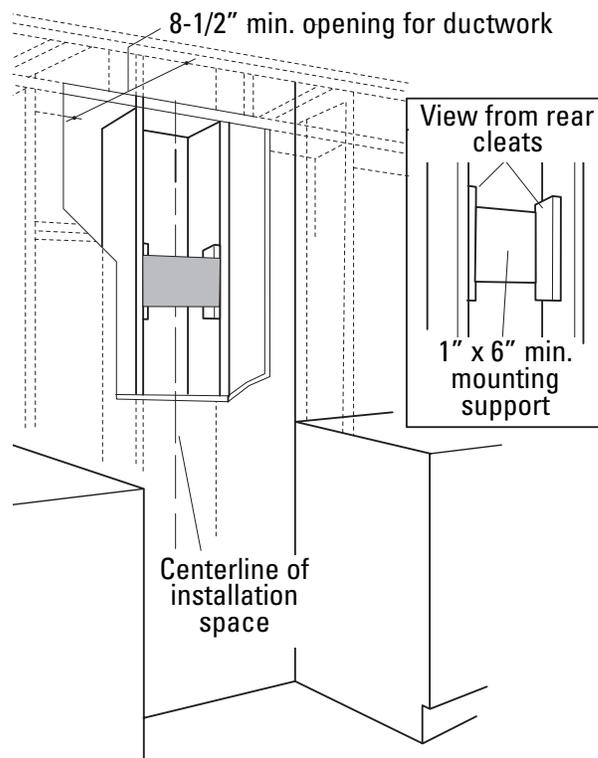
If drywall is present, mark the screw hole locations for the top mounting brackets. Remove the template.
