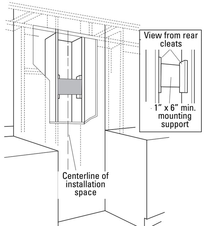
If drywall is present, mark the screw hole locations for the top mounting brackets. Remove the template.
