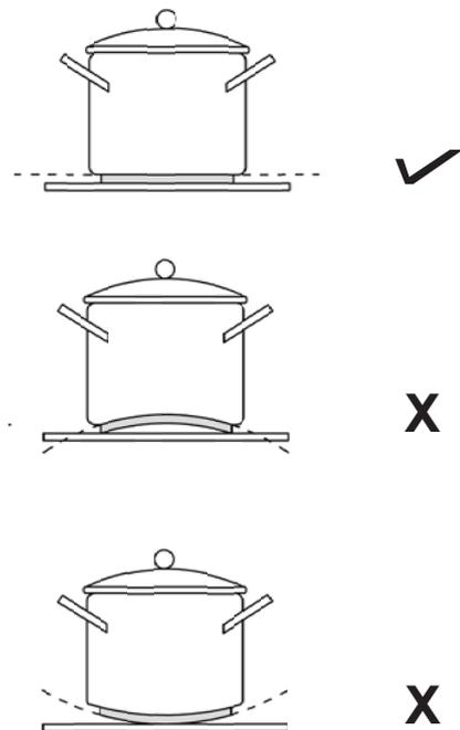
The pans must have certain minimum diameter to ensure optimal operation. Pans larger than the cooking zones can also be used: make sure that the bottom of the pan does not touch other cooking zones and that it is always centered over the inductor.
