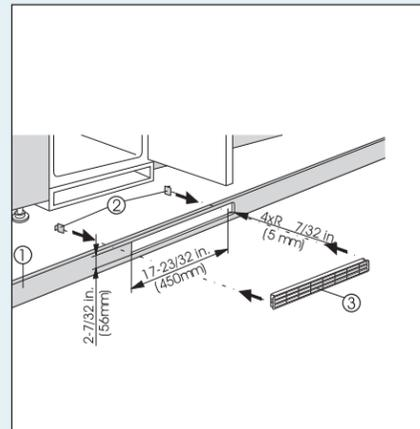
Ventilation through the cabinet base at the bottom can be achieved by installing the provided ventilation grille (3) or via a ventilation opening of at least 31 in.<sup>2</sup> (200 cm<sup>2</sup>).
