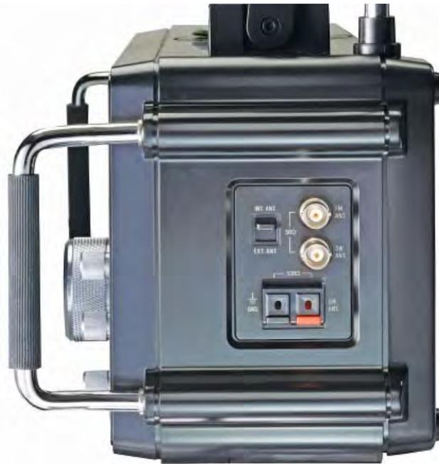
**Figure 9** — The Etón Elite 750's external antenna connectors.
