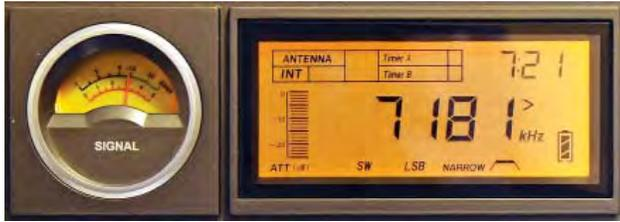
Figure 7 — The Elite 750 S-meter and display.
