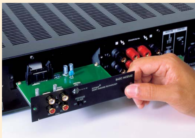
Smart Amplifier Technology (SAT) gives you outstanding flexibility to upgrade or outfit your system simply by inserting a new module.
