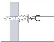
Tap EZ anchor tip into marked drywall locations, turn with screwdriver until seated flush.
