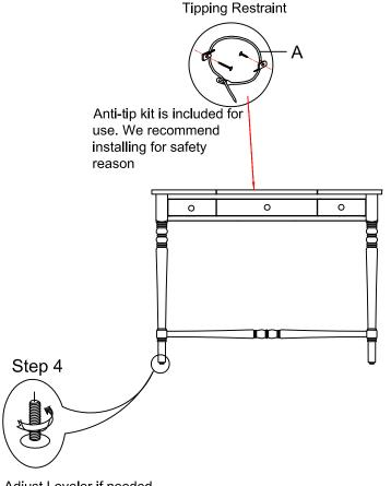
Adjust Leveler if needed to level case on uneven floor.
