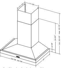
Install hood so that the bottom of the unit is 24" to 30" above the cooking surface. Mounting height may be affected by ceiling height.
