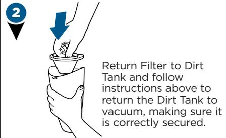
**NOTE:** After heavy usage, you may clean the Filter by washing it gently by hand in warm water and mild dish detergent. Rinse thoroughly and make certain it is completely dry before replacing it. If filter is torn, replace it with a new filter.
