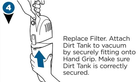
**NOTE:** The Dirt Tank may be rinsed with warm water and a mild detergent if needed. The Dirt Tank must be thoroughly dried before replacing.
