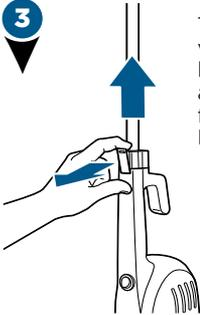
To use as a hand vacuum, release the latch from the Handle and pull Handle away from the machine. Press the latch closed.
