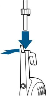
To use as a floor vacuum, open the latch at the top of the Hand Vacuum Grip and insert Handle. Once Handle is all the way inserted into the body of the vacuum, press the latch closed to secure the Handle in place.
