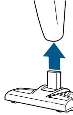
Then, attach the floor nozzle by inserting it into the opening at the bottom of the Dirt Tank. Press firmly to secure in place.
