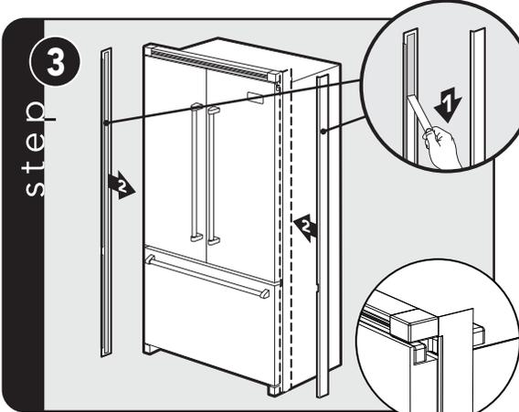
Shim trim has adhesive backing on both sides. Remove adhesive backing on refrigerator side only. Fit the shim trim to the front of the unit first. With center hinge, the shim trim will have a cutout. Use the cutout to locate the height of the shim trim.
