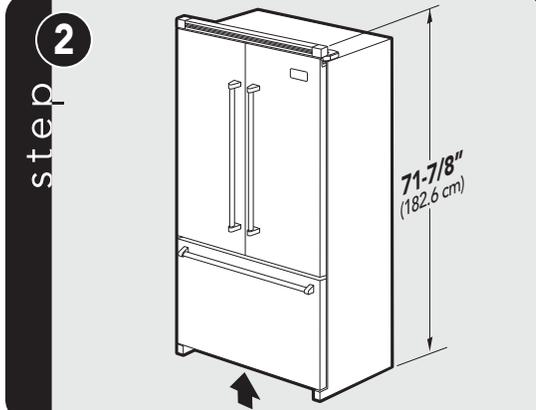
Raise the unit up until the measurement from the floor to the top of the grille assembly is 71-7/8 inches.
