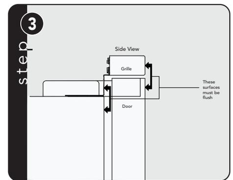
Align and position grille on top of unit so that the face of the grille and the face of the door are flush.
