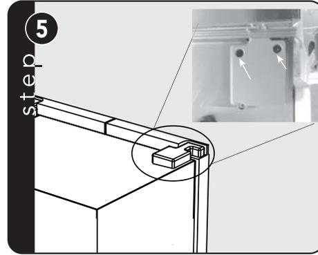
Place plastic caps back on top of hinges and located existing holes. Insert screws making sure the grille is centered.
