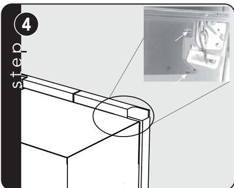
Use the two inner hole locations to properly align the grille.
