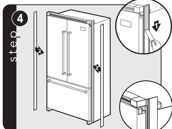
Remove adhesive backing for the side trim. Locate the top of the side trim with the top of the grille assembly. Press the side trim into the refrigerator cabinet at the center location.
