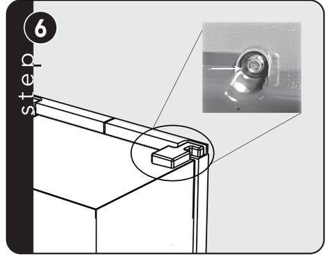
Use washer when replacing screw in rear hole of plastic cap. Tighten all hex screws
