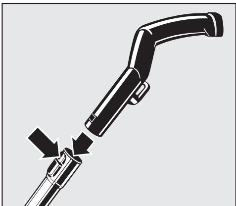
The handle can also be fitted directly to the vacuum housing.
