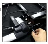
B.Re-insert the pin and R clip with actuator bracket. Repeat for foot actuator.
