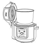
**3** Make sure the pressure release valve is in the SEAL position.
